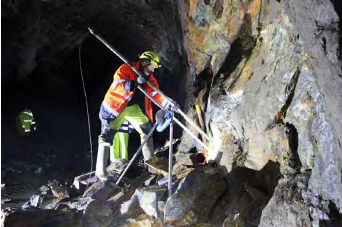
Figure 1: Borehole logging in the Wolfsberg underground exploration mine in Austria by the GREENPEG partner terratec Geophysical Services GmbH.
