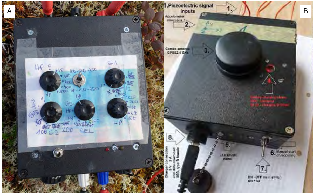
Figure 2: A) Specialized amplifier for piezoelectric signals and B) the first prototype for the GREENPEG piezoelectric seismograph.
