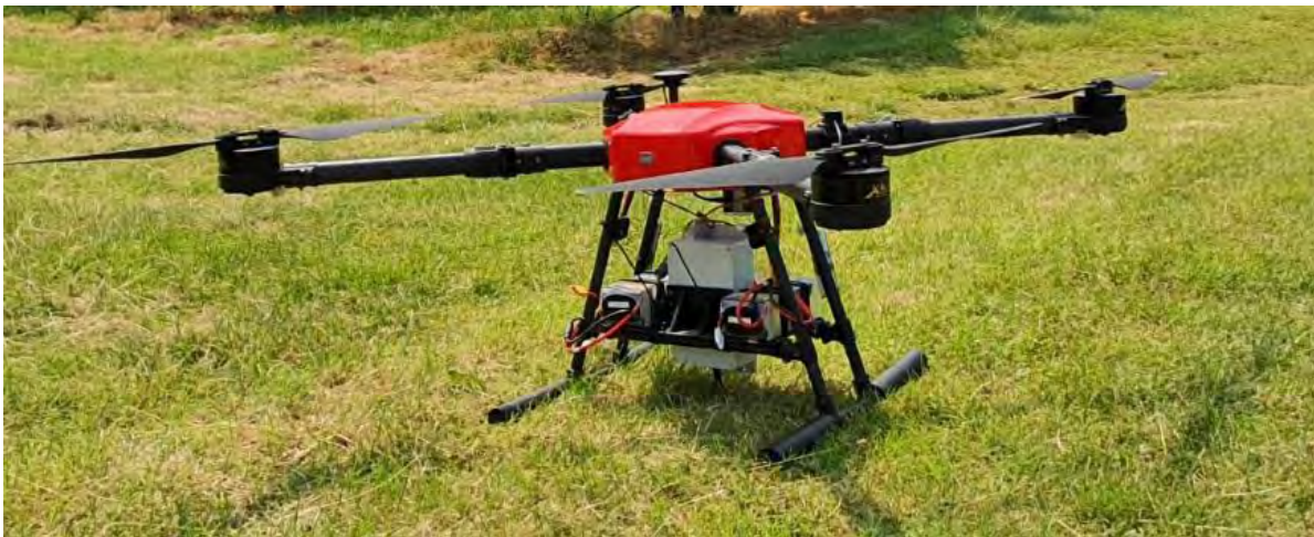
Figure 2: Drone-borne acquisition system with equipped hyperspectral camera
